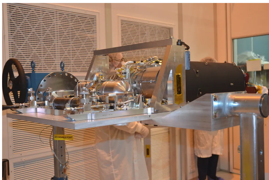
Figure 1. JWST's MIRI instrument cryocooling system. Image credit: NASA/JPL, reproduced from [16].
